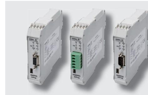
The fieldbus modules enable direct connection to the PLC. Configuration is done with the bus configurator. No more than 1 fieldbus module can be connected to the base module via the T connector on the rear side of the module. The status of fieldbus modules are displayed via the LED's on the front of each module.
