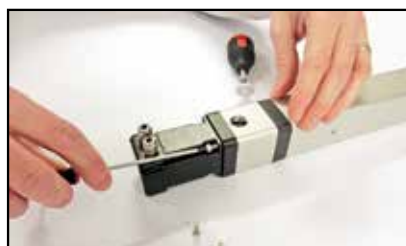
Tighten motor mounting screws
