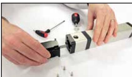
Insert motor shaft into coupling
