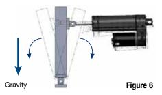
**No Meter Out**: In this case the load is unaffected by acceleration of gravity. There is no need to control the load because it is controlled by an external means. Select metering code "N"
