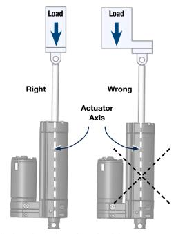
Loads should act along the axis of the actuator. Off-center loads may cause binding and lead to premature unit failure.
