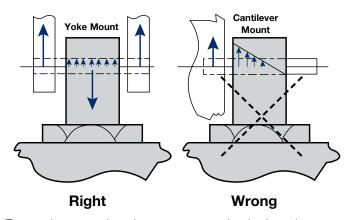
Ensure that mounting pins are supported at both ends. Cantilevered mounting is unacceptable. Failure to provide proper support will shorten unit life.
