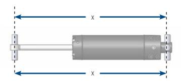
Mounting pins must be parallel to each other as shown above. Pins which are not parallel can cause excess vibration or actuator binding.
