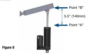
**Example (Figure 9):** 5.5" (140mm) of travel required to move the load from point A to point B. Select an H-Track with 6" (152mm) of stroke.
