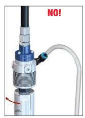
**WHAT'S WRONG:** Drain line points up, which can flood the union's bearings.
