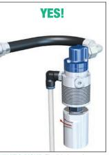
WHAT'S RIGHT: Flexible hose between rigid supply pipe and union. Drain hose runs straight down.
