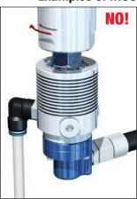
WHAT'S WRONG: Union points up. Coolant contaminants will collect at the bottom and interfere with proper sealing.
