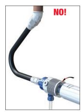
WHAT'S WRONG: Bend in supply hose is too tight. When pressurised, the supply hose may create a large side load on the union's bearings.
