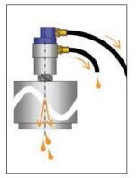
When the supply line runs down from the rotating union, any coolant between union and control valve will remain in the hose during tool change. This reduces the amount of drainage from both the spindle nose and the union drain line.
