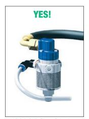
WHAT'S RIGHT: Elbow fitting is used to avoid a tight bend in supply hose. Drain hose slopes downward.
