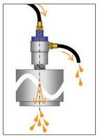
When the supply line runs up from the rotating union, any coolant between union and control valve will flow down during tool change. This increases the amount of drainage from both the spindle nose and the union drain line.
