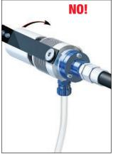
WHAT'S WRONG: Union housing is rigidly attached to the spindle. Without 100% perfect alignment, this creates a side load leading to early bearing failure.
