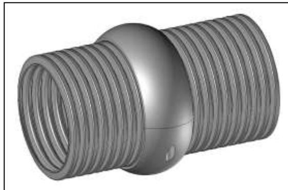
Protectors as shock- and abrasion protection for wellpipes with G-profile in NW95. PAPRB-90 is a standard protector, which is also suitable for combination or for repair of wellpipes. In the Combi-Protector-System the protectors are connected by the connecting element VAKEM, to lead wellpipes parallel. Also the combination with different nominal widths is possible. With screw closure.
