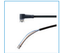
Plug-in connector Angled Cable 5m - Socket M8 (female) KAW500
